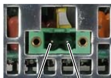
Figure 6-2 Connecting the device to the 24 VDC power supply
