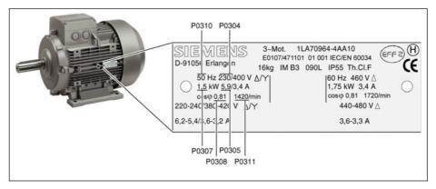
Figure 3-6 Typical Motor Rating Plate Example
