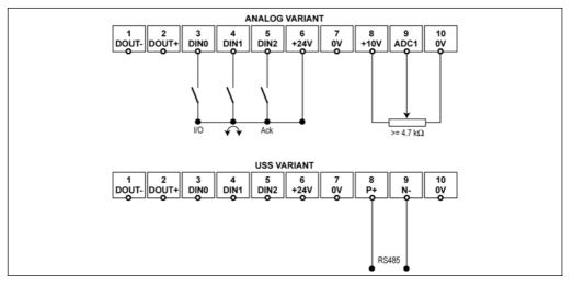
Figure 3-3 Basic operation – Analog and USS Variants
