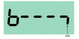
5. The lower mark on the right-hand side of the display indicates that DIN0 is active high, that is, an ON command is present.
