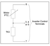
Figure 3-7 Motor Overload PTC
