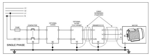
Figure 2-7 Motor and Power Connections
