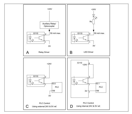
Figure 3-8 Typical Configurations of the Digital Output
