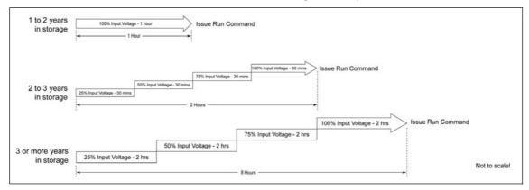
Figure 2-1 Reforming Capacitors After a Period of Storage
