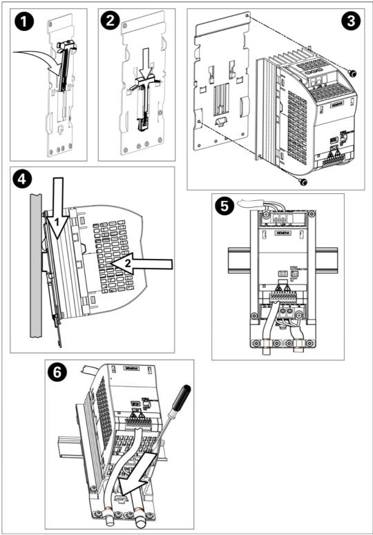
4. Holding the front of the inverter, pull the inverter forward and upwards to release it from the DIN rail.
