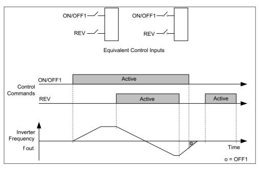
Figure 4-1 Siemens standard control using ON/OFF1 and REV
