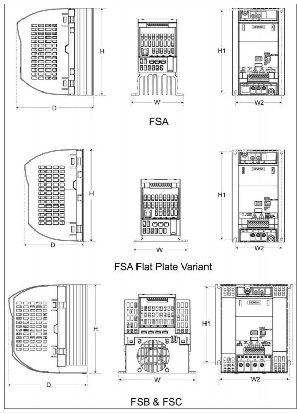
Figure 2-3 Dimensions of the SINAMICS G110
