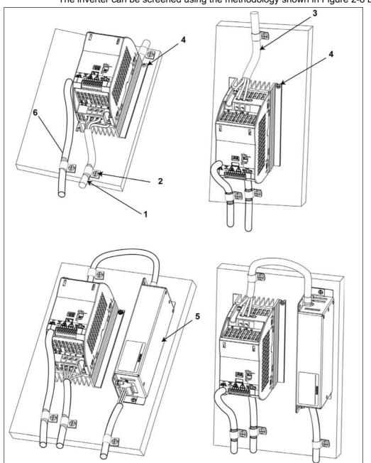
The inverter can be screened using the methodology shown in Figure 2-8 below.
