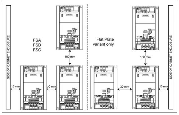
Figure 2-4 Clearance distances for mounting the inverter
