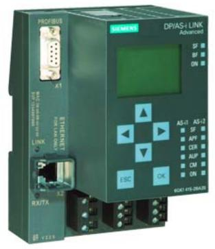
SIMATIC NET, DP/AS-INTERFACE LINK ADVANCED; GATEWAY PROFIBUS DP/AS-INTERFACE WITH MASTER PROFILE M3, M4 ACC. TO EXTENDED AS-I SPEC. V3.0 FOR INTEGRATION IN PROFIBUS DP; DOUBLE MASTER WITH DISPLAY; DEGREE OF PROTECTION IP20.
