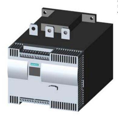
SIRIUS soft starter Values at 400 V, 40 °C Standard: 313 A, 160 kW Inside-delta: 542 A, 315 kW 200-460 V AC, 230 V AC Screw terminals
