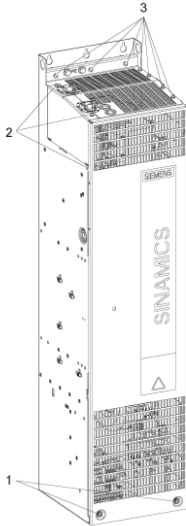
Figure 3-4 Installing the Braking Module in a Power Module, frame size FX – steps 1 - 3
