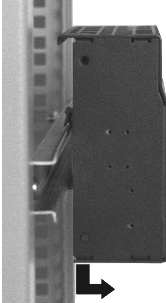
Figure 4. Removing from the Standard Rail
