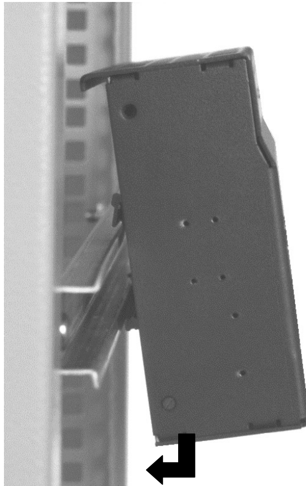
Figure 3: Installing the OMC on a DIN Standard Rail
