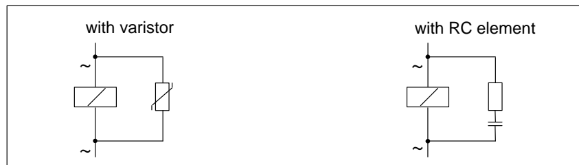
Figure 4-9 Suppressing AC-Operated Coils
