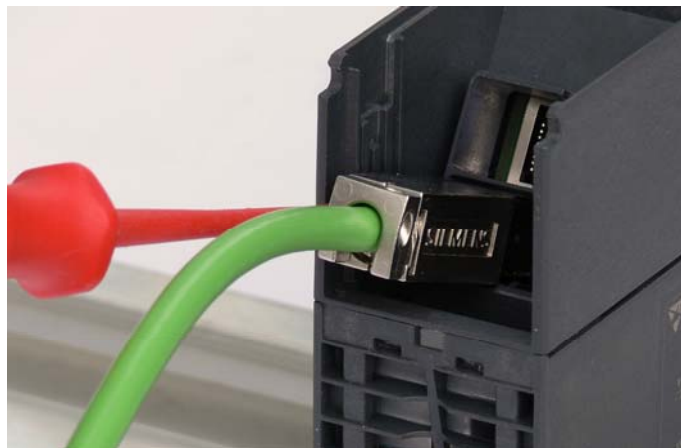
Figure 4-7 Removing the IC FC RJ-45 Plug by releasing the RJ-45 Plug using a screwdriver
