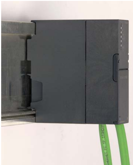
Figure 4-1 CSM 377 installation on a SIMATIC S7-300 standard rail
