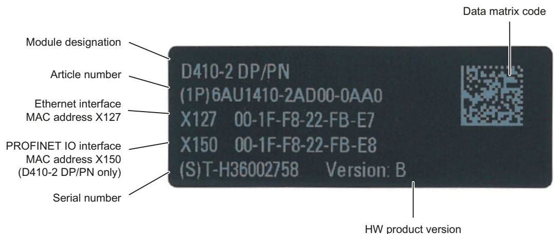
Figure 2-9 SIMOTION D410-2 DP/PN MAC addresses
