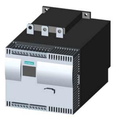
SIRIUS soft starter Values at 400 V, 40 °C Standard: 113 A, 55 kW Inside-delta: 196 A, 110 kW 200-460 V AC, 230 V AC Screw terminals
