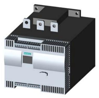
SIRIUS soft starter Values at 400 V, 40 °C Standard: 250 A, 132 kW Inside-delta: 433 A, 250 kW 200-460 V AC, 230 V AC Screw terminals
