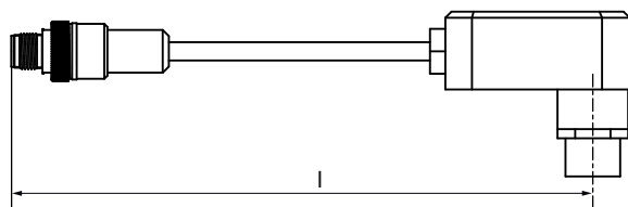
Figure 13-1 Connecting cable, M12 ↔ Reader / SLG; l = 2 m, 5 m (MOBY U)
