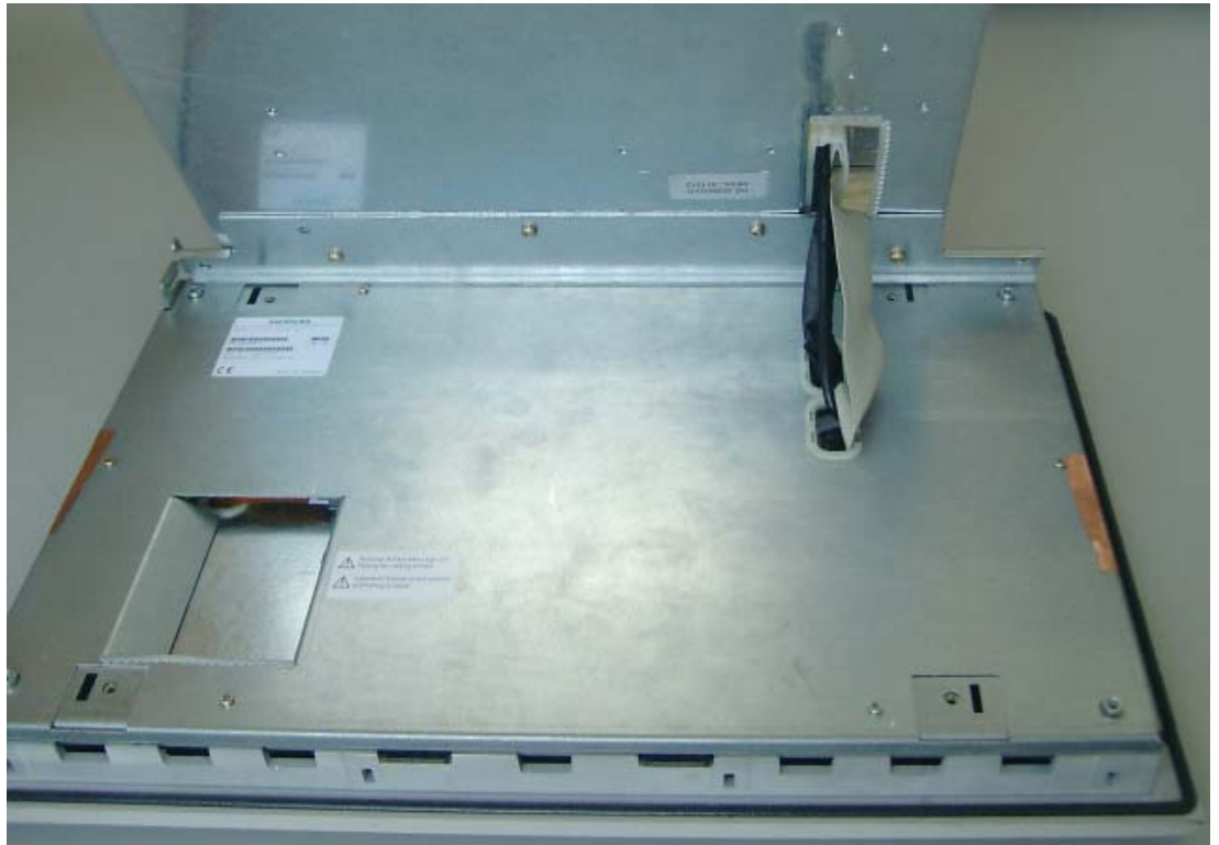
Figure 10-17 Separating from the control unit from the computer unit, ribbon cable
