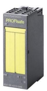
SIMATIC DP, POWER MODULE PM-E F PROFISAFE, FOR ET 200S; 24V DC USEABLE FOR INSTALLATIONS WITH UNGROUNDED REFERENCE POTENTIAL RELAIS FOR FAIL-SAFE SWITCHING OF VOLTAGE BUSES P1 AND P2 UP TO CATEGORY 3 (EN954-1)/ SIL2 (IEC61508)/PLD (ISO13849), 2 FAIL-SAFE DIGITAL OUTPUTS UP TO CATEGORY 4 (EN954-1)/ SIL3 (IEC61508)/PLE (ISO13849), ALSO USEABLE IN PROFINET-NETWORKS W. IM151-3 HF
