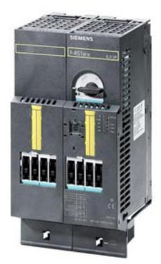
F-RS1E-X FOR ET 200S FAILSAFE REVERSING STARTER SETTING RANGE 0.3...3A MECHANICAL SWITCHING ELECTRONIC PROTECTION AC-3, TO 1.1KW/400V, CAN BE EXPANDED FOR BRAKE CONTROL MODULE FOR 2DI CONTROL MODULE
