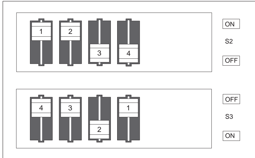
Figure 4-6 Standard Settings of Switches S2 (1 to 4) and S3 (1 to 4) for 333 MHz Pentium PII CPU
