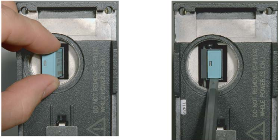
Figure 4-2 Inserting the C-PLUG in the device and removing the C-PLUG from the device with a screwdriver
