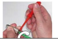
Insert a 2.5 mm screwdriver into the hole in the locking mechanism and continue turning it as far as the limit stop.
