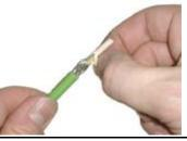
If the white filler was not pulled off when you stripped the cable, remove it and the transparent protective foil manually. Cut off the dummy cores.
