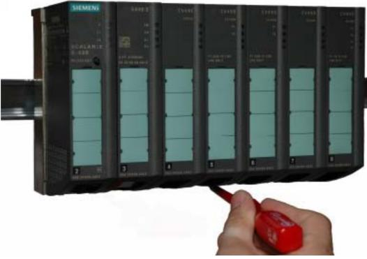
Figure 6-38 Removing the SCALANCE X408-2 from a 35 mm DIN rail
