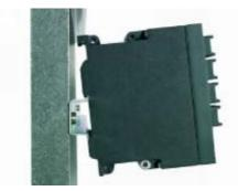
Figure 6-7 SCALANCE X-100 removing from a DIN rail (35 mm)
