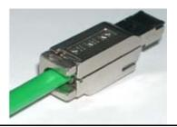
The connector is correctly locked when the opening of the locking mechanism is at the side and the side edges are flush with the connector.
