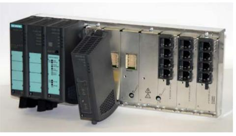
Figure 6-58 Inserting a media module
