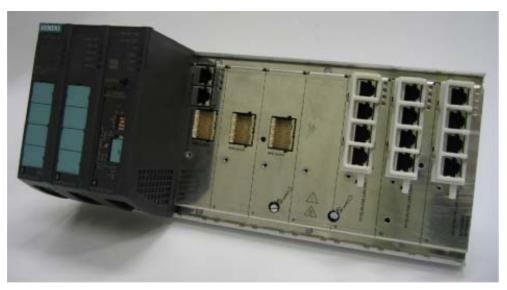
Figure 6-32 Basic device without media modules, protective caps and covers
