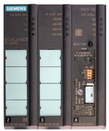
Figure 6-39 Power module, digital inputs and CPU module with operator controls on the SCALANCE X414-3E
