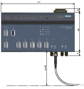
Figure 9-7 Industrial Ethernet OSM ITPxx (dimensions in mm)
