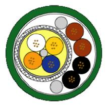
Figure 10-6 Structure of the IE Hybrid Cable
