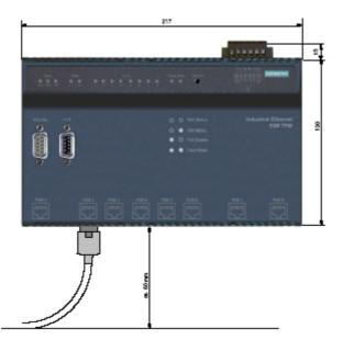
Figure 9-11 Industrial Ethernet ESM TP80 (dimensions in mm)
