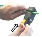
Place the cable in the stripping tool. The index finger of your left hand is the limit stop.
