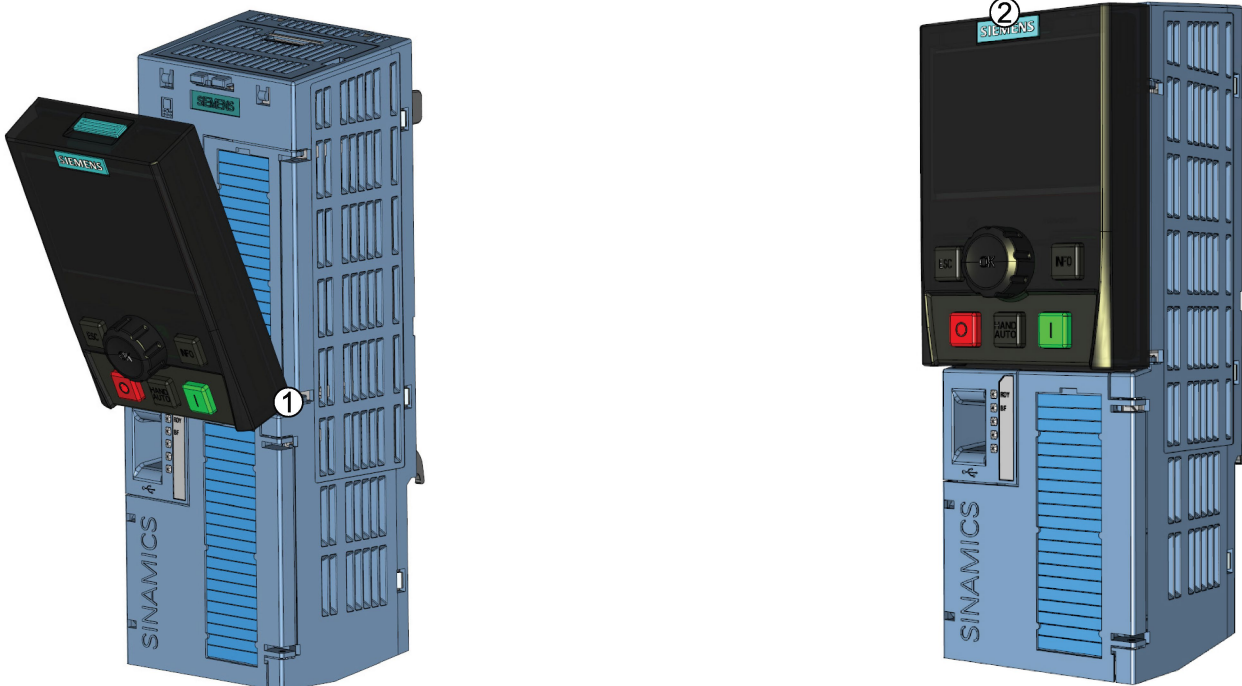
Figure 3-1 Fitting the IOP to the Control Unit
