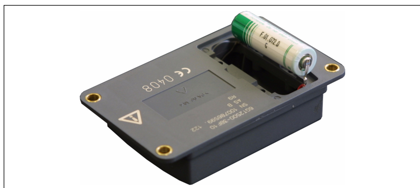
Figure 3-13 Open MDS with battery pulled out
