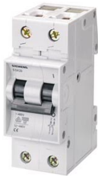
CIRCUIT BREAKER T55 400V, 6KA, 2-POLE, D, 6A
