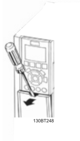
Figure 5.37: Access to control terminals for A2, A3, B3, B4, C3 and C4 enclosures
