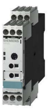
Timing relay, multifunction Phase-out product! For further information, contact our sales department 2 CO contacts, 16 functions 15 time ranges (0.05 s-100 h) 24 V, 200-240 V AC and 24 V DC at 50/60 Hz AC with LED, screw terminal
