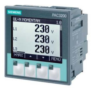
SENTRON, measuring instrument, 7KM PAC3200, LCD, L-L: 690 V, L-N: 400 V, MODBUS TCP, optional Modbus RTU / PROFINET / PROFIBUS, apparent / active / reactive energy, Cl. 0.5 acc. to IEC61557-12 or Cl. 0.5S acc. to IEC62053-22, Wide-voltage power supply unit, AC/DC, screw connection
