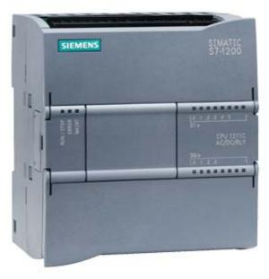
\*\*\* SPARE PART\*\*\* SIMATIC S7-1200, CPU 1211C, COMPACT CPU, AC/DC/RELAY, ONBOARD I/O: 6 DI 24V DC; 4 DO RELAY 2A; 2 AI 0 - 10V DC, POWER SUPPLY: AC 85 - 264 V AC AT 47 - 63 HZ, PROGRAM/DATA MEMORY: 25 KB
