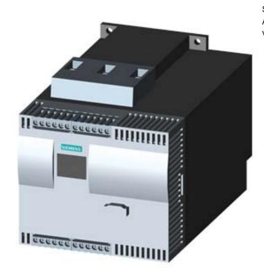
SIRIUS soft starter Values at 400 V, 40  $^\circ C$  Standard: 29 A, 15 kW Inside-delta: 50 A, 22 kW 200-460 V AC, 230 V AC Screw terminals
