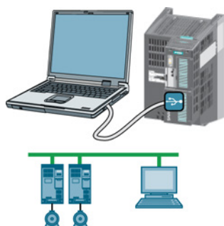
Figure 7-3 Connection using the PC connection kit
