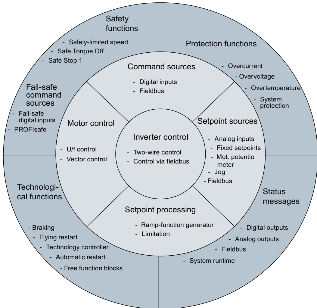
Figure 7-1 Overview of inverter functions
