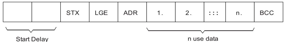
Figure 6-18 Structure of USS telegram
