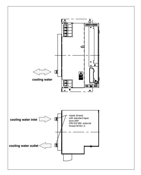
Cooling water connection, PSI 6300.XXX W1/W2
