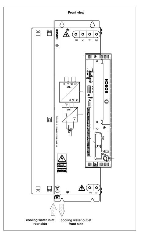
Cooling water connection, PSI 6200.XXX W1/W2
