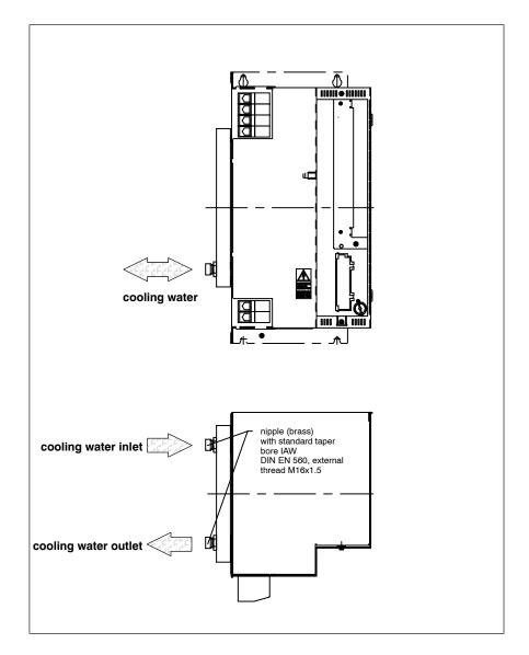
Cooling water connection, PSI 6100.XXX W1/W2
