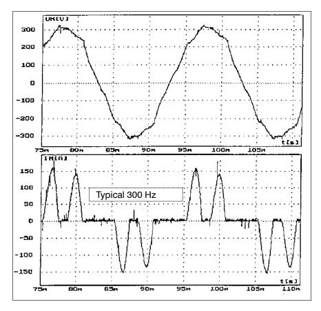
The 5th, 7th, 11th, 13th, 15th, and 17th harmonic wave are the characteristic harmonics of the mains current curve. The harmonic component depends on the welding power.
