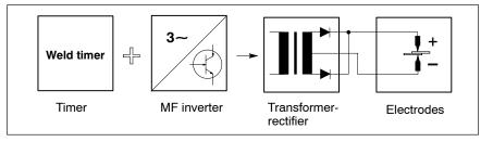
Basic functional design of the 1 kHz MF welding process
