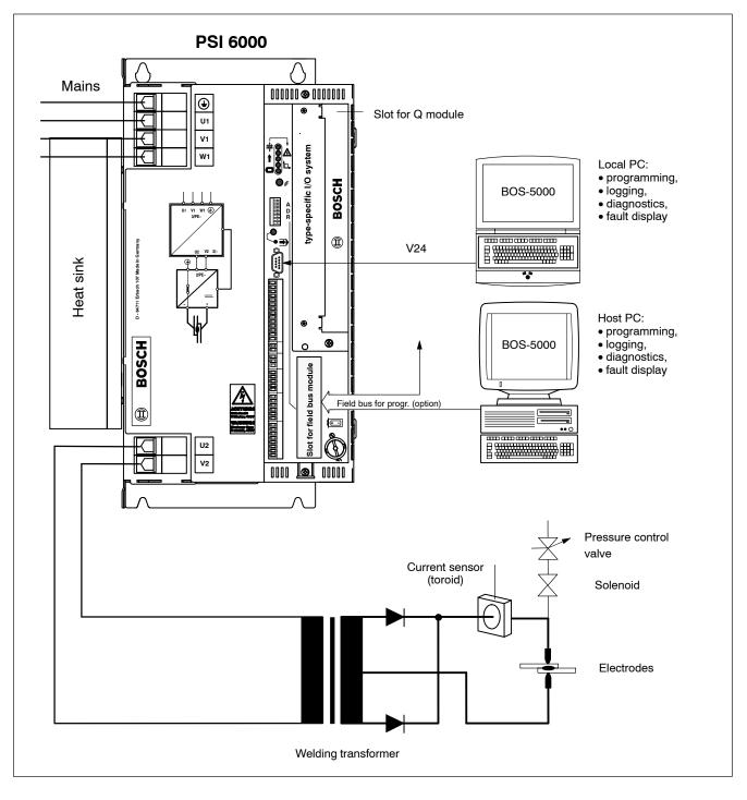
Setup for welding
