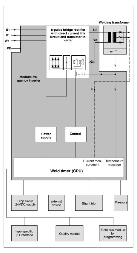
Block diagram of a medium-frequency inverter
