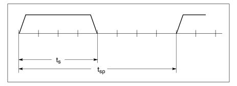
Weld time and overall weld cycle duration
