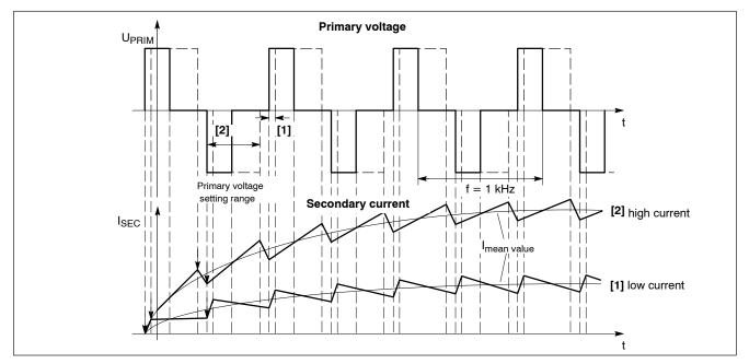
Primary and secondary voltages for medium-frequency welding
