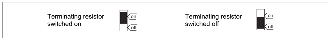
Figure 7-10 Terminating resistor switched on and off
