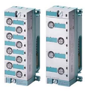
SIMATIC DP, ELECTRONIC MODULES FOR ET200PRO 4 DO DC 24V, 2.0A HIGH FEATURE, CHANNEL DIAGNOSTICS; SHORT CIRCUIT AND WIRE BREAK; INCLUSIVE BUS MODULE CONNECTING MODULE IO 6ES7194-4..00-0AA0 MUST BE ORDERED SEPERATELY
