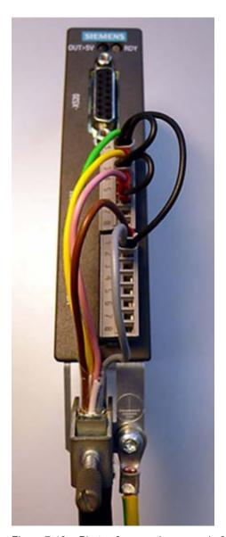
Figure 7-13 Photo of connection example 2: SMC30, 30 mm wide
