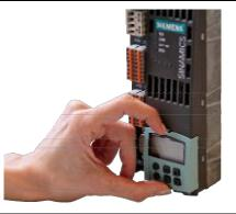
4. Press the latching cams on the BOP20 together simultaneously and push the BOP20 straight into the housing of the CU305 until you hear it latch into position.
