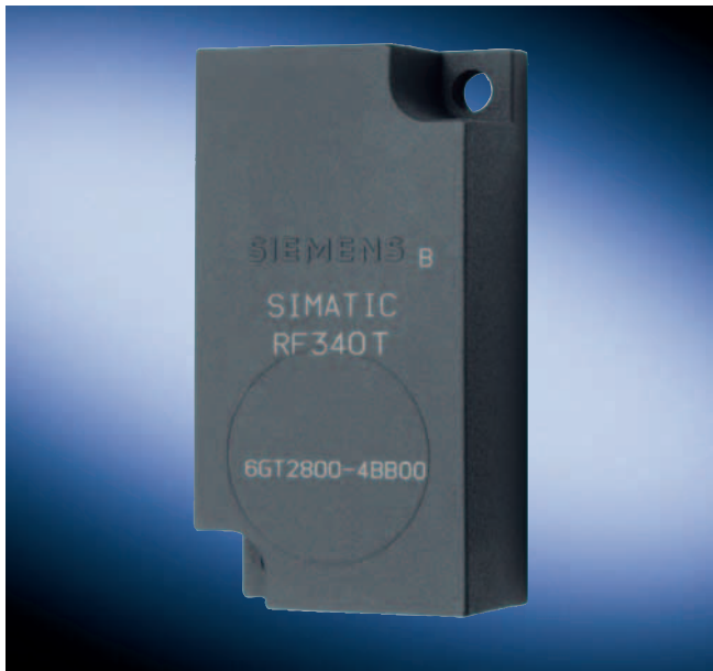
Universal data memory (8 KB FRAM + 24 byte EEPROM + 4 byte serial number), particularly suitable for small workpiece carriers.
