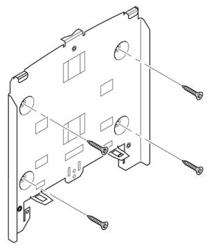
Figure 5-8 Fitting the mounting plate for the SCALANCE W786 to a wall
