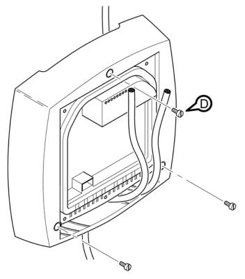
Figure 5-14 Screwing a SCALANCE W786 to a mounting plate
