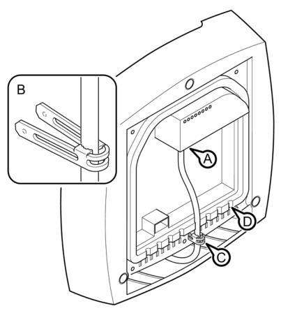
Figure 6-1 Connecting a cable and fitting the strain relief clamps
