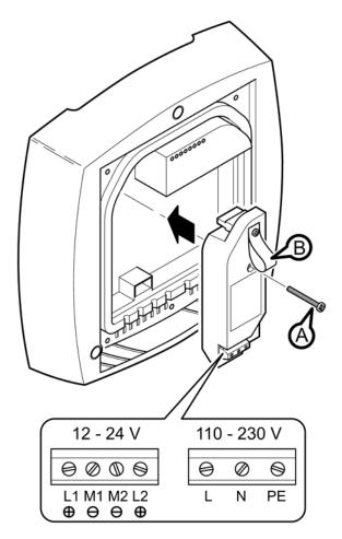
Figure 6-6 Using a power supply adapter in a SCALANCE W786
