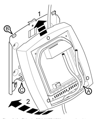
Figure 5-13 Fitting the SCALANCE W786 to a mounting plate
