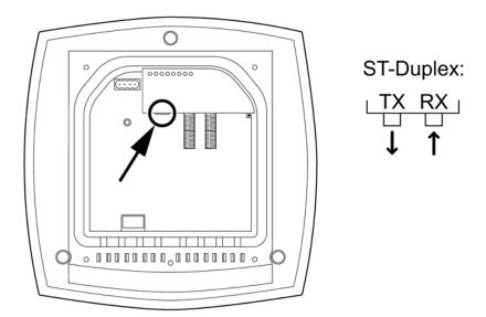
Figure 6-7 Position of the Ethernet port with the housing cover removed
