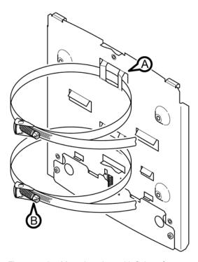
Figure 5-12 Mounting plate with fittings for mast mounting
