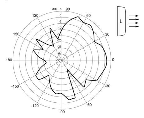
7.4 Radiation patterns diagrams of SCALANCE W786 internal antennas
