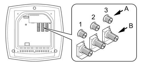
Figure 6-8 Position of the ports for external antennas with the housing cover removed
