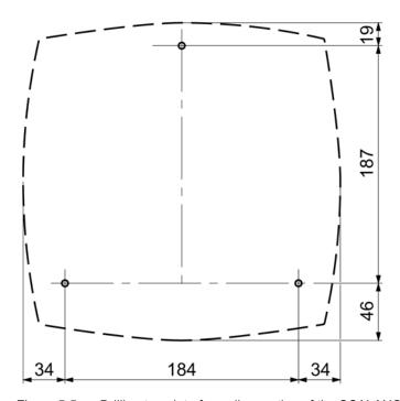
Figure 5-5 Drilling template for wall mounting of the SCALANCE W786
