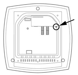
Figure 4-2 Position of the reset button with the housing cover removed
