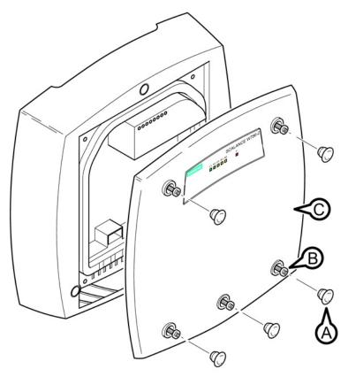
Figure 5-1 Removing the cover A Sealing cap B Cover screw C Housing cover
