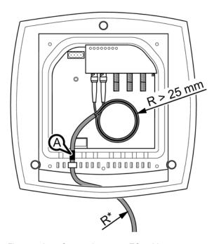
Figure 5-3 Connecting up an FO cable
