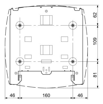
Figure 5-7 Drilling template for fitting the mounting plate to a wall
