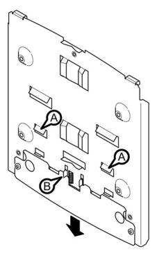
Figure 5-11 Mounting plate with fittings for DIN rail mounting
