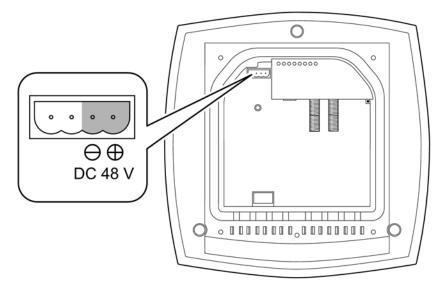
Figure 6-4 Position of the opening in the housing for the power supply with the housing cover removed
