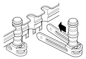
Figure 6-2 Securing a sealing plug with a strain relief clamp
