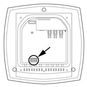
Figure 6-9 Location of the C-PLUG with the housing cover removed
