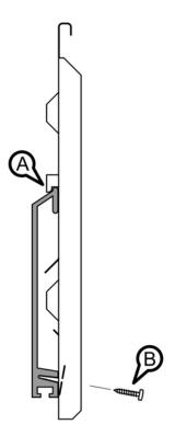
Figure 5-10 Side view of a mounting plate on an S7-300 standard rail
