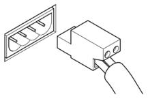
Figure 6-5 Position of the connector when inserted in the socket of the housing
