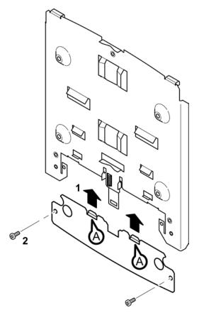
Figure 5-9 Fitting and securing the cover plate for the cable feedthrough
