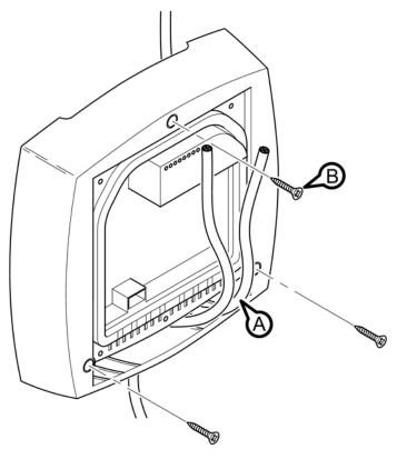
Figure 5-6 SCALANCE W786 wall mounting
