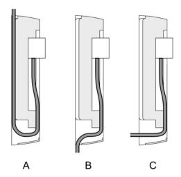
Figure 5-2 Side view of a SCALANCE W786 with cables entering from different directions
