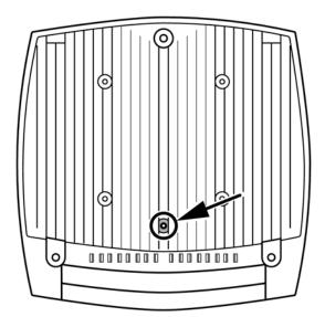
Figure 5-4 Chassis ground connector on the rear of the SCALANCE W786
