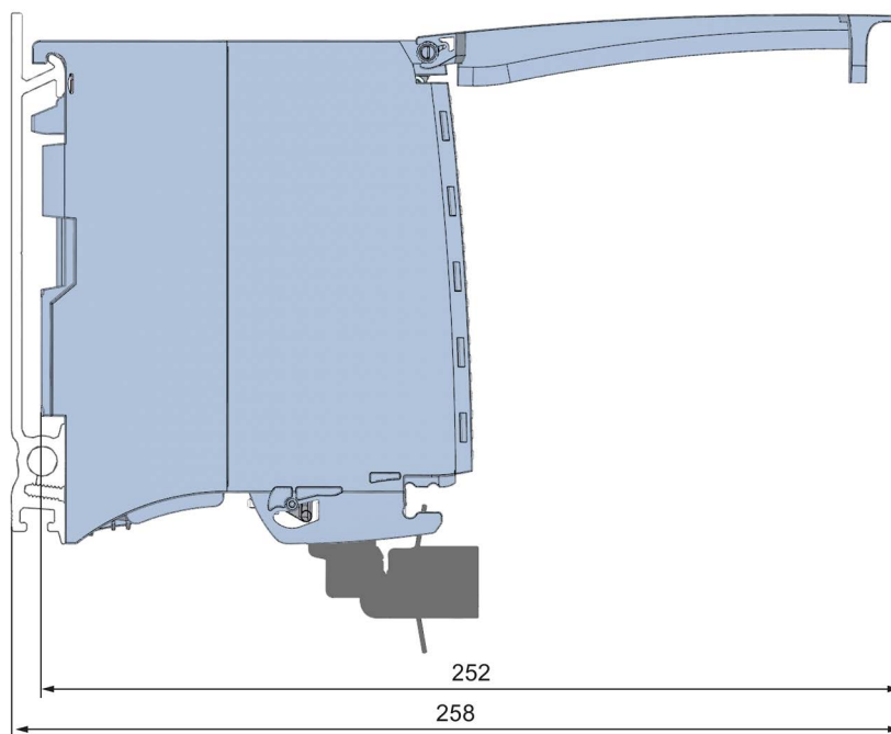
Figure A-2 Dimensional drawing of the AQ 8xU/I HS module, side view with open front panel
