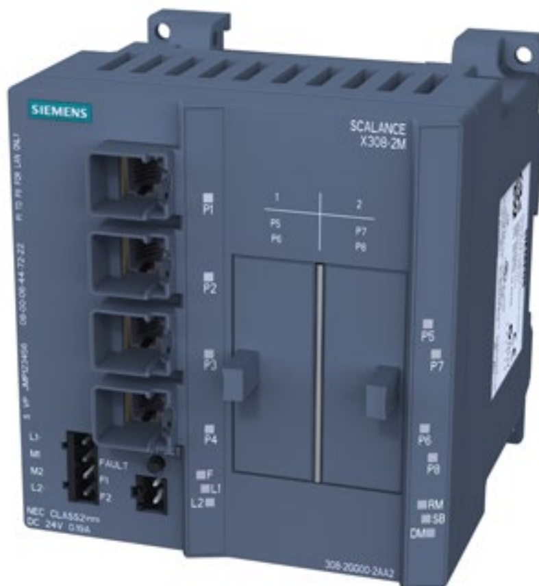
Figure 4-13 SCALANCE X308-2M with dummy covers
