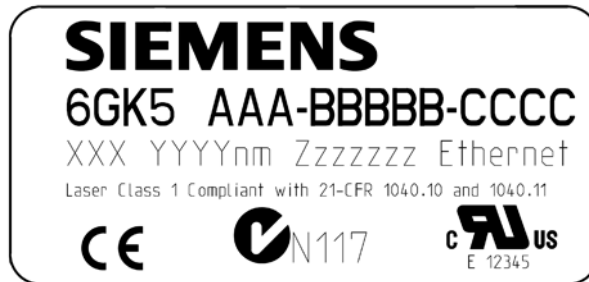
Figure 9-8 SFP specimen type plate top
