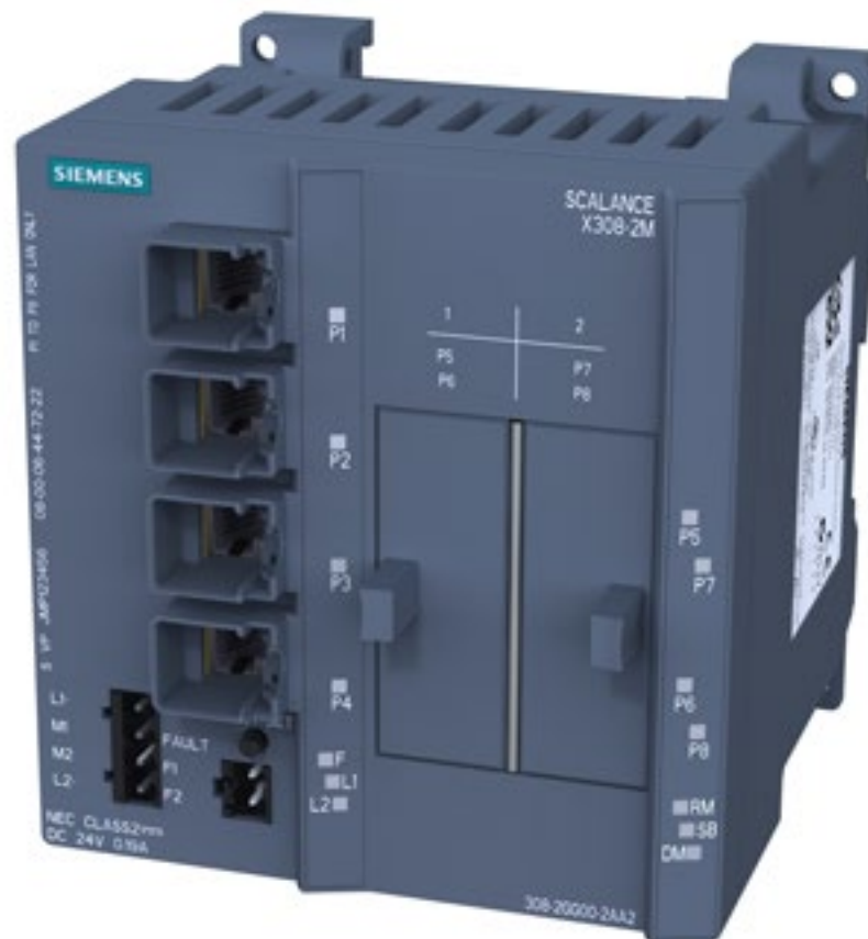
Figure 4-22 SCALANCE X308-2M PoE with dummy covers
