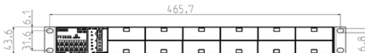
Figure 11-10 Front view of the XR324-12M
