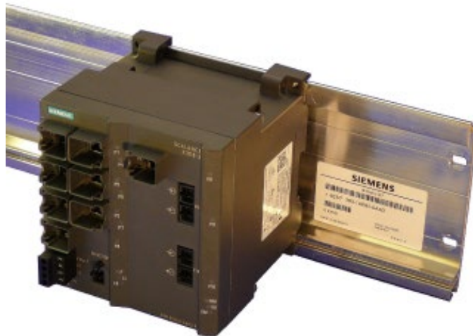
Figure 5-2 Installing an IE Switch X-300 on a SIMATIC S7-300 standard rail
