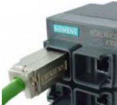
Figure A-2 Inserting the IE FC RJ-45 Plug (based on the example of the IE FC RJ-45 Plug 180)
