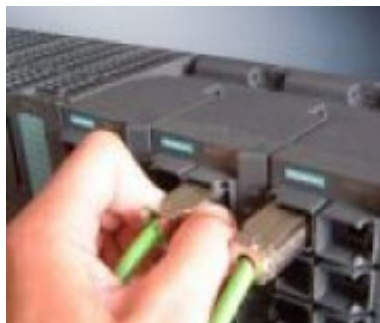
Figure A-3 Releasing the RJ-45 plug (based on the example of the IE FC RJ-45 Plug 180)
