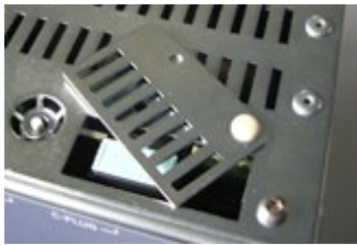
Figure 4-18 C-PLUG of the X-300EEC
