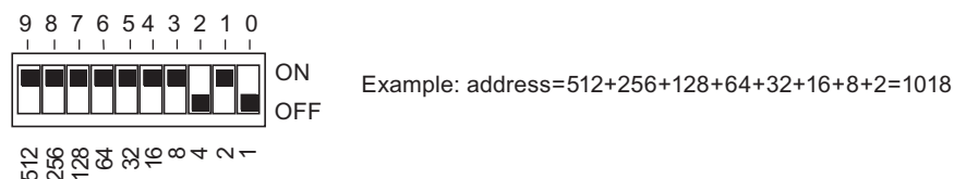
Figure 3-1 Example for Setting the Address Switch (DIP Switch)
