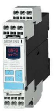
DIGITAL MONITORING RELAY FOR THREE-PHASE LINE VOLTAGE AUT. CORRECTION OF PHASE SEQUENCE PHASE FAILURE 3X 160 TO 690V AC 50 TO 60 HZ UNDERVOLT. AND OVERVOLT. 160-690V HYSTERESIS 1-20V OFF DELAY 0-20S 1 W FOR POWER SYSTEM FAULTS 1W FOR PHASE CORRECTION SPRING-LOADED TYPE
