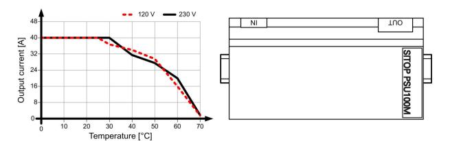
Figure 4-23 6EP1337-3BA00 mounting position (3)
