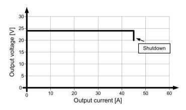
Figure 6-17 6EP1337-3BA00 latching shutdown output characteristic
