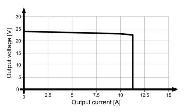
Figure 6-11 6EP1334-3BA10 parallel operation output characteristic
