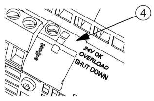
Figure 2-6 Status indicators and signals (example of 6EP1337-3BA00)
