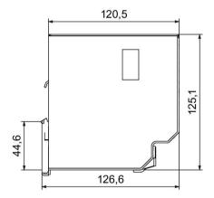
Figure 2-13 Dimension drawing for 6EP1336-3BA00
