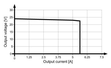
Figure 6-10 6EP1333-3BA10 parallel operation output characteristic
