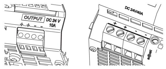
Figure 5-2 Output connection (example, 6EP1334-3BA10 and 6EP1337-3BA00)
