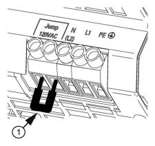
Figure 2-9 Wire jumper (example, 6EP1437-3BA00)
