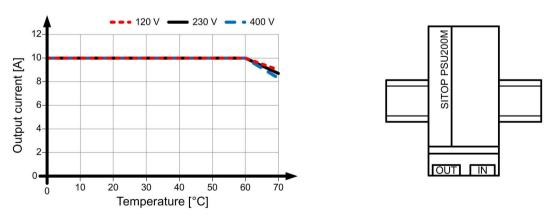
Figure 4-2 6EP1334-3BA10 output current for a standard mounting position
