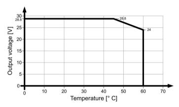
Figure 6-7 Output derating depending on the ambient temperature at Iout rated
