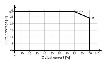
Figure 6-8 Output derating depending on the output current at  $60^{\circ}$  C
