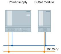
Figure 9-6 Buffering brief power failures using the SITOP PSE201U buffer module
