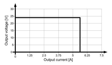
Figure 6-3 6EP1333-3BA10 single operation output characteristic
