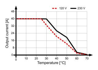
Figure 4-22 6EP1337-3BA00 mounting position (2)
