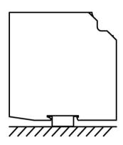
Figure 4-9 6EP1333-3BA10 mounting position (4)
