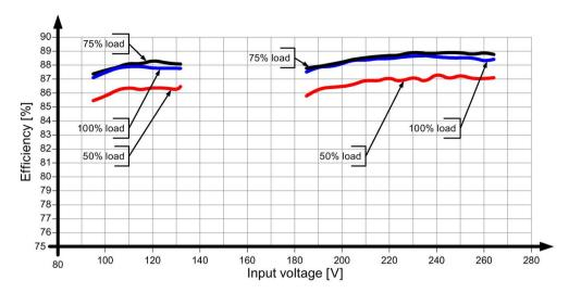
Figure 6-20 6EP1336-3BA00 efficiency
