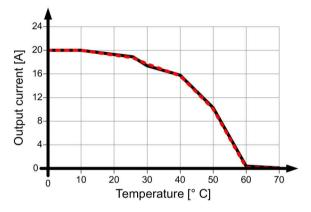
Figure 4-20 6EP1336-3BA00 mounting position (5)
