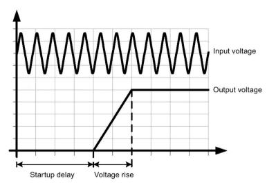
Figure 6-2 Startup delay/voltage rise
