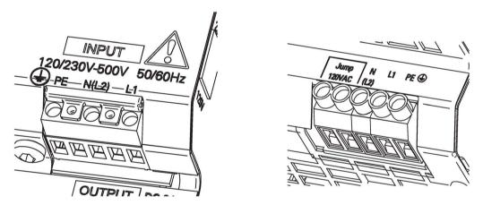
Figure 5-1 Line connection (example, 6EP1334-3BA10 and 6EP1337-3BA00)
