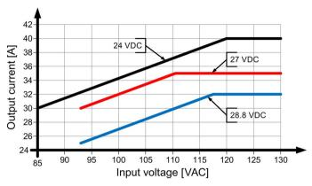
Figure 6-9 Output derating depending on the input voltage
