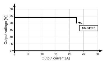
Figure 6-16 6EP1336-3BA00 latching shutdown output characteristic
