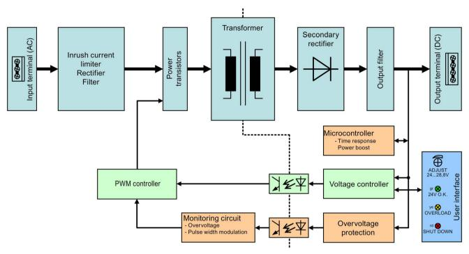
Figure 2-11 Block diagram for 6EP1336-3BA00 and 6EP1337-3BA00
