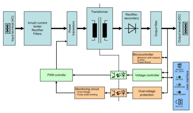
Figure 2-10 Block diagram for 6EP1333-3BA10 and 6EP1334-3BA10
