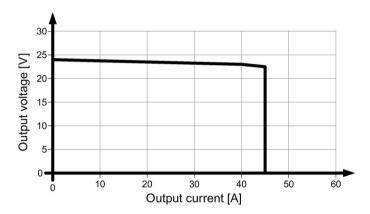
Figure 6-13 6EP1337-3BA00 parallel operation output characteristic
