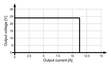
Figure 6-4 6EP1334-3BA10 single operation output characteristic
