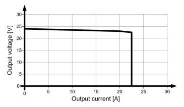
Figure 6-12 6EP1336-3BA00 parallel operation output characteristic
