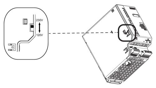
Figure 2-8 Voltage selector switch (example, 6EP1334-3BA10)
