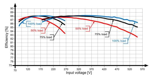
Figure 6-18 6EP1333-3BA10 efficiency
