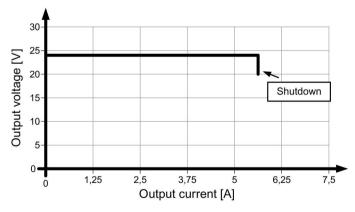
Figure 6-14 6EP1333-3BA10 latching shutdown output characteristic
