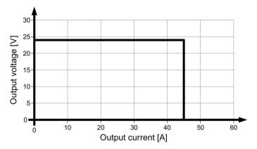
Figure 6-6 6EP1337-3BA00 single operation output characteristic
