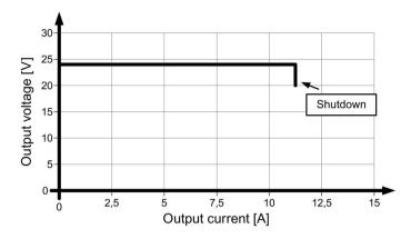
Figure 6-15 6EP1334-3BA10 latching shutdown output characteristic
