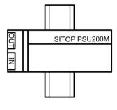
Figure 4-7 6EP1333-3BA10 mounting position (2)
