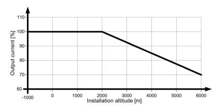
Figure 4-5 Mounting height derating
