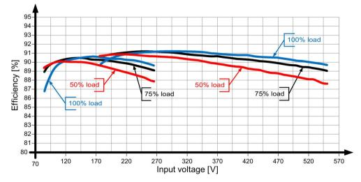
Figure 6-19 6EP1334-3BA10 efficiency
