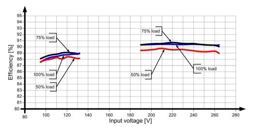
Figure 6-21 6EP1337-3BA00 efficiency
