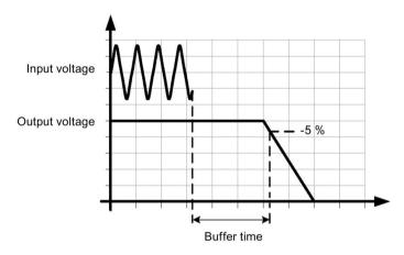
Figure 6-1 Power-failure buffering
