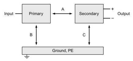
Figure 7-1 Test voltage diagram
