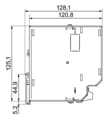
Figure 2-14 Dimension drawing for 6EP1337-3BA00
