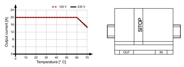
Figure 4-3 6EP1336-3BA00: Output current in the standard mounting position
