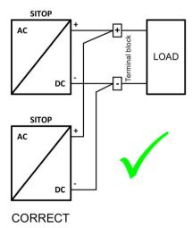
Figure 9-1 Parallel connection
