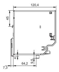
Figure 2-12 Dimension drawing, 6EP1333-3BA10 and 6EP1334-3BA10 (example, 6EP1334-3BA10)
