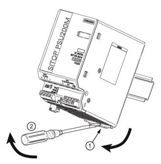
Figure 3-1 Removal (example, 6EP1334-3BA10)
