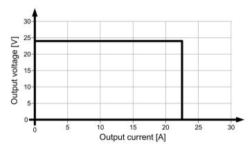
Figure 6-5 6EP1336-3BA00 single operation output characteristic
