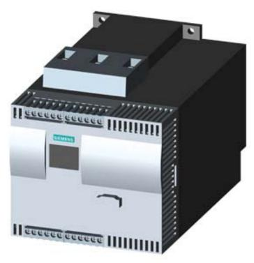
SIRIUS soft starter Values at 400 V, 40  $^{\circ}$ C Standard: 93 A, 45 kW Inside-delta: 161 A, 90 kW 200-460 V AC, 230 V AC Screw terminals
