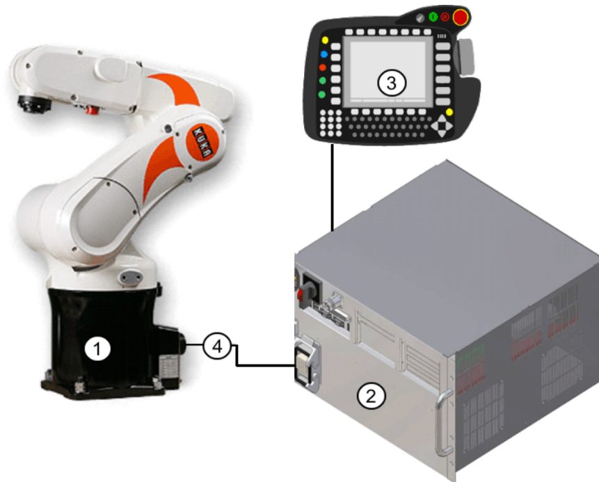
Fig. 1-1: Example of an industrial robot
