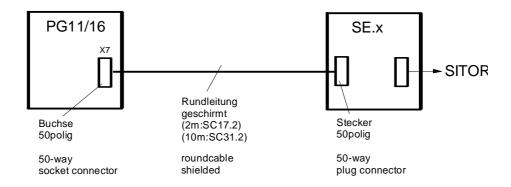
The SITOR interface is simulated in the interface board SE20. This is required when connecting a SITOR cubicle system which does not have it's own interface. The output of the current actual value, in analog form, to the test jack X13 and X5 pin 6 is then no longer required.
