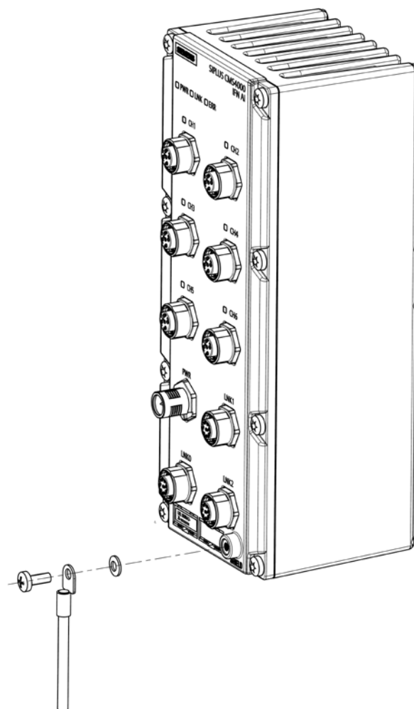
Picture 8 Connecting IFN AI to the ground (SHIELD)
