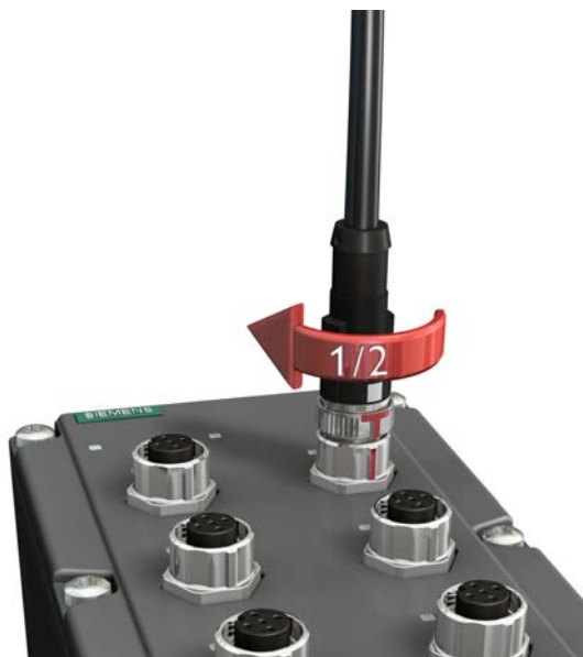
Picture 10 M12-socket plug interlocking
