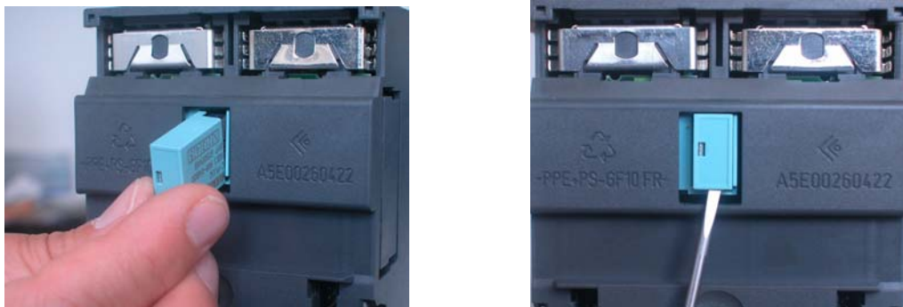
Figure 3-2 Fitting a C-PLUG in the IE/PB Link PN IO and Removing a C-PLUG from the IE/PB Link PN IO using a Screwdriver
