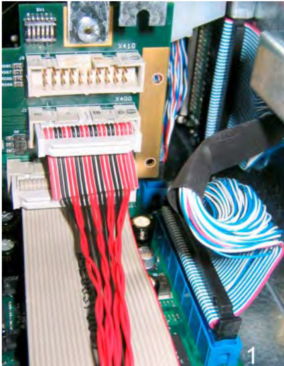
Figure 10-12 Ribbon cable and IDE cable on the motherboard
