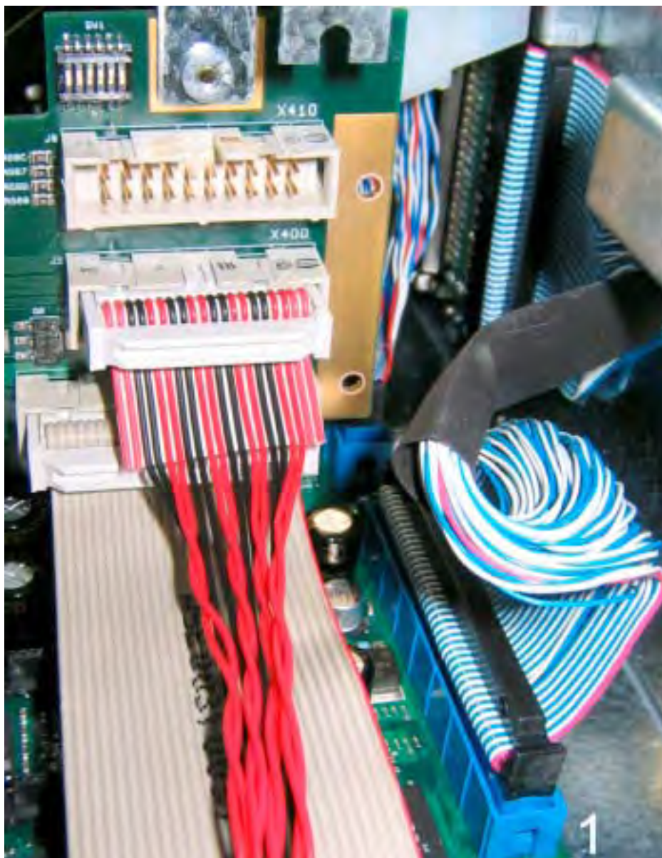
Figure 10-6 Ribbon cable and IDE cable on the motherboard
