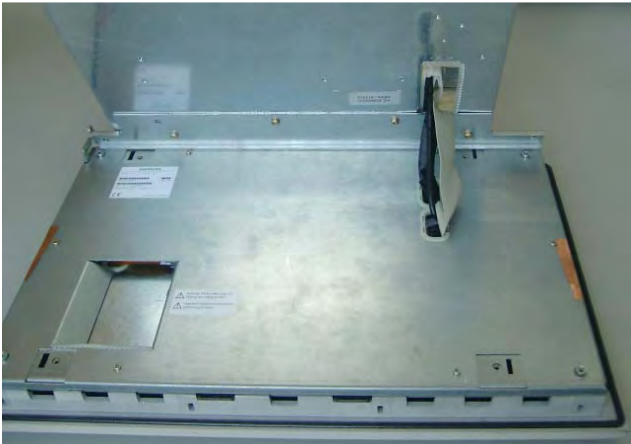
Figure 10-17 Separating the control unit from the computer unit, ribbon cable
