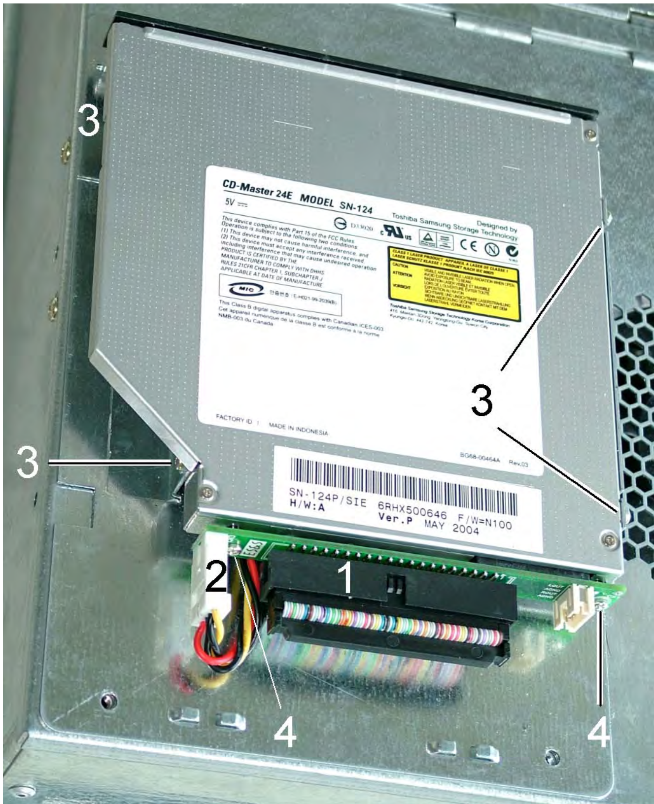
Figure 10-4 Drive without housing
