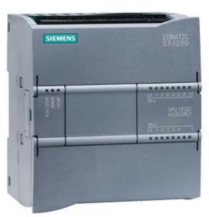
\*\*\* SPARE PART\*\*\* SIMATIC S7-1200, CPU 1212C, COMPACT CPU, AC/DC/RLY, ONBOARD I/O: 8 DI 24V DC; 6 DO RELAY 2A; 2 AI 0 - 10V DC, POWER SUPPLY: AC 85 - 264 V AC AT 47 - 63 HZ, PROGRAM/DATA MEMORY: 25 KB
