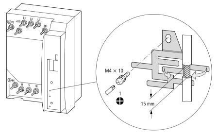
Figure 45: Connecting the screen of the control signal cables
