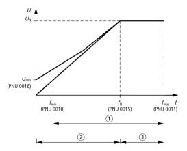
Figure 33: Usable motor speed range
