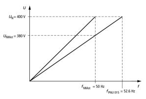
Figure 32: Calculation of characteristic point PNU 015
