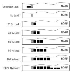
Figure 48: Motor load display
