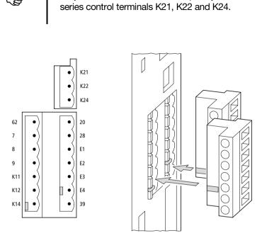
Figure 44: Inserting the plug-in terminals for the control signals
