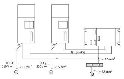
Figure 22: Earthing when a PLC is used
