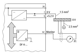
Figure 28: Connecting a meter to the monitor signal
