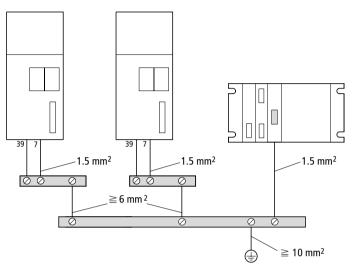
Figure 20: Earthing with star arrangement
