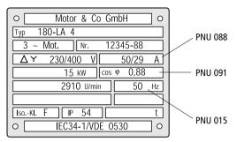
Figure 34: Motor name plate
