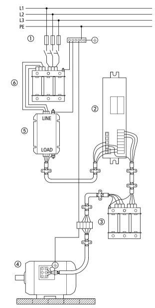
Figure 4: Overview of screening measures and installation
