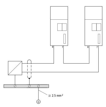
Figure 27: Master setpoint input with current loop signal
