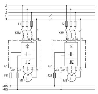
Figure 16: Single-phase AC main feed with interconnected DC bus
