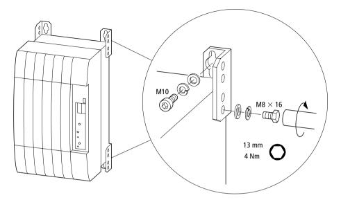
Figure 42: Fixing to the mounting plate (DF4-341-45K to 90K)
