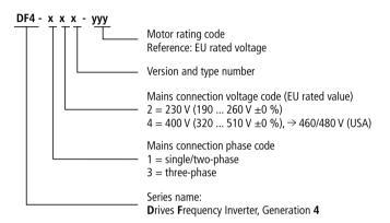
Figure 1: Structure of type code
