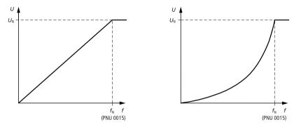
Figure 30: Linear and quadratic frequency response
