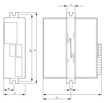
Figure 49: Dimension drawing of DF4-120/340
