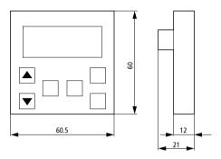
Figure 51: Dimension drawing of LCD keypad
