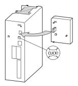
Figure 46: Plugging in the LCD keypad
