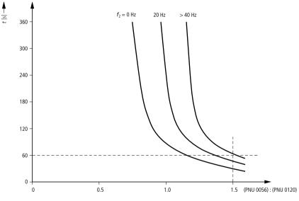
Figure 36: I<sup>2</sup>t monitoring
