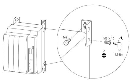
Figure 41: Fixing to the mounting plate (DF4-341-15K to 30K)
