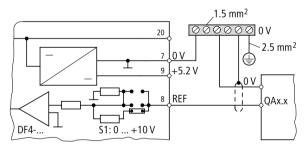
Figure 24: Setpoint entry from a PLC
