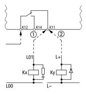
Figure 29: Relay connection for DC or AC circuit
