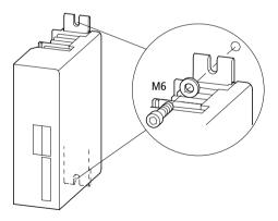
Figure 40: Attaching to the mounting plate
