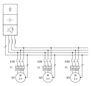
Figure 14: Parallel connection of several motors
