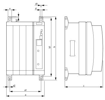
Figure 50: Dimension drawing of DF4-341
