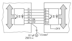
Figure 21: Interconnection with a PLC
