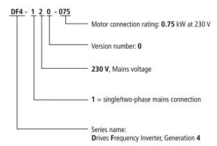
Figure 2: Type code for frequency inverters
