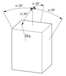
Figure 38: Mounting angle for DF4 series
