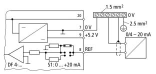
Figure 26: Analog setpoint with current loop signal
