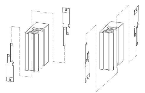
Figure 39: Inserting the mounting rails
