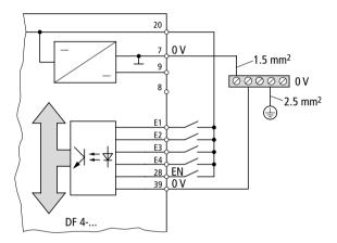
Figure 19: Earthing of 0 V potential
