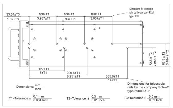
Figure 14-2 Dimensional drawing for the use of telescopic rails
