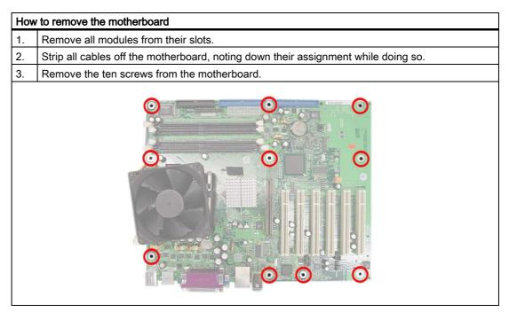
A replacement motherboard is supplied without processor and memory modules.
