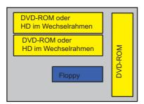
Figure A-3 Approved configuration versions for the temperature range 5 to 40° C
