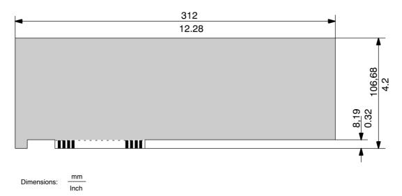
Figure 14-3 Long format PCI module
