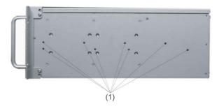
Position of the mounting holes (1) for angle brackets or telescopic rails
