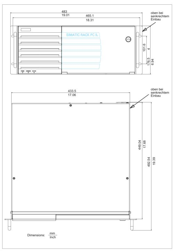
Figure 14-1 Dimensional drawing of the device
